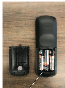
Insert (3) AAA Alkaline Batteries
