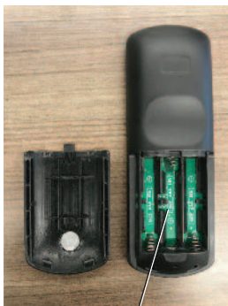
Polarity Markings Inside the Battery Compartment
