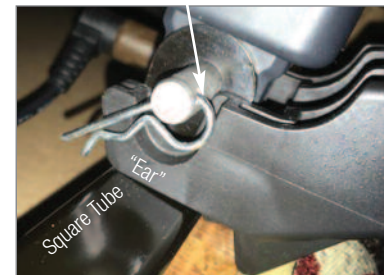
Arrow Shows “Ear” Stopping on Motor Pin
