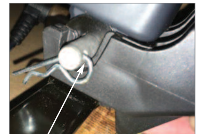
Arrow Shows Motor Pin is ALL the way to the back of the “Ear”
