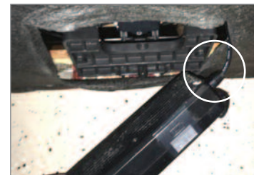
Connect Motor Connector Directly to the Power Supply for Sectional and Chair Styles
