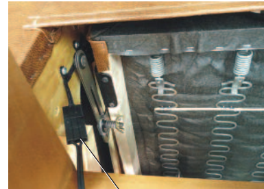
Thermo-Electric Cooler Power Transformer Connection
